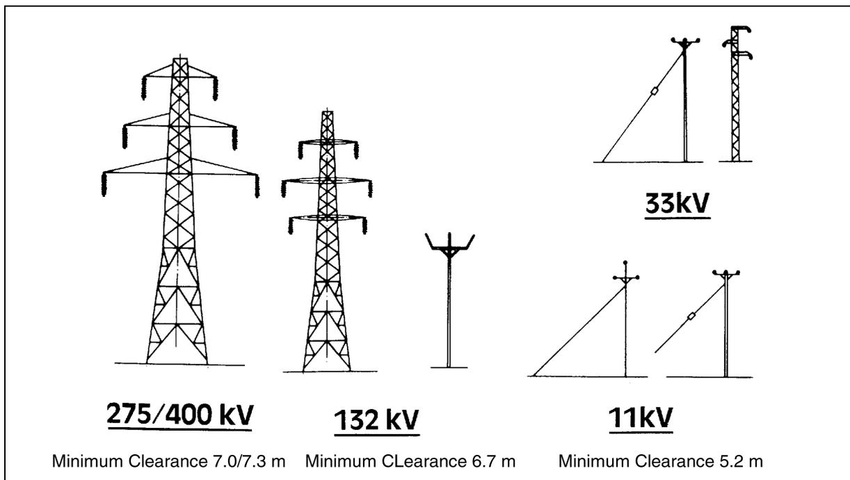
**Figure 1** Typical Overhead Line Supports
